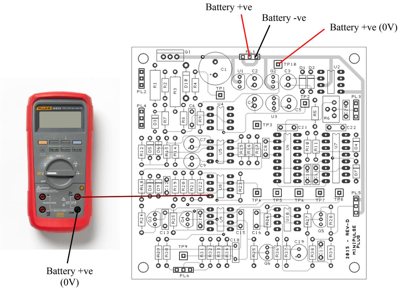
Fig. 2: Checking the - 5V Supply
