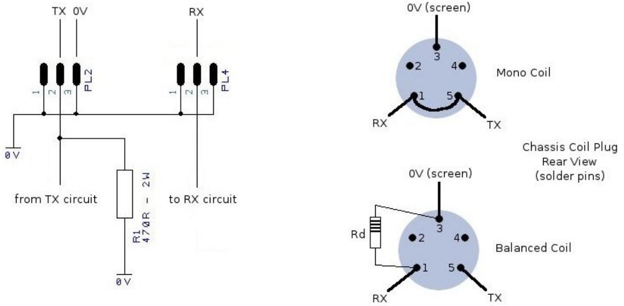
Fig. 7: Coil Configurations
