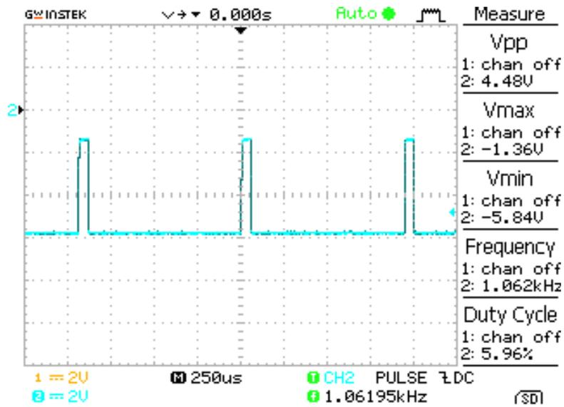
Fig. 5: TX Oscillator Waveform
