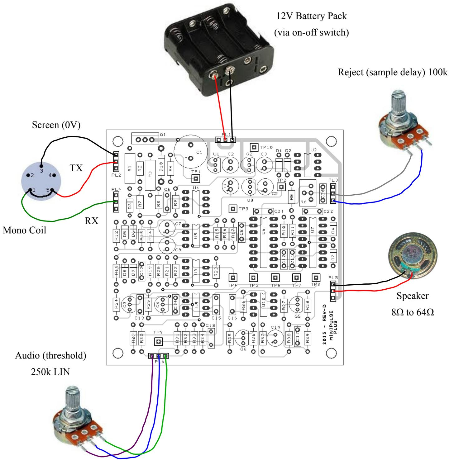
Fig. 14: PCB External Connections
