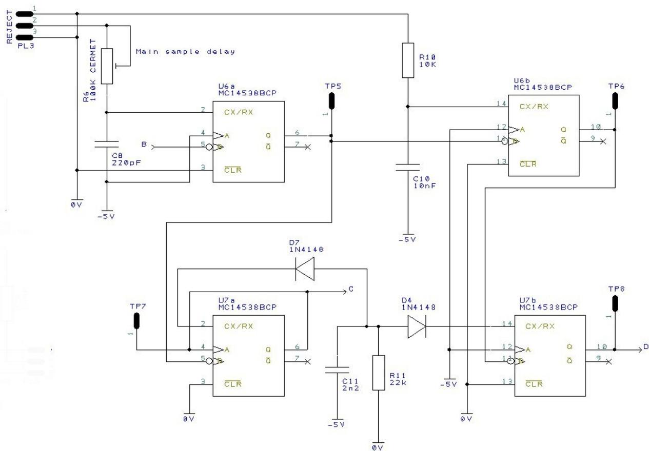
Fig. 9: Sample Pulse Generator
